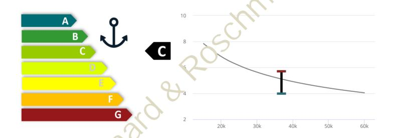
The VESSELINDEX®- GHG rating reflects to what extent the normal operational span, ie. 11 to 14 knots for handysize, of the vessel is vithin the current IMO compliance limit (represented by the gray line).
